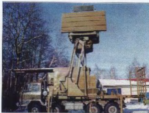
3D-Central Acquisition Radar (3D-CAR)
